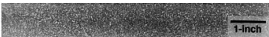
Figure 6b - A transverse section of a 7xxx alloy with Al-3%Ti-0.15%C at 30% of the normal Ti addition level showing no TCG. Etch: Fennell's reagent.
