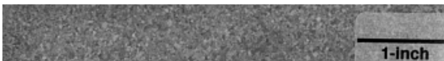
Figure 5b - A transverse section of a 7xxx continuously cast plate with Al-6%Ti-0.02%C addition. Etch: Fennell's reagent.
