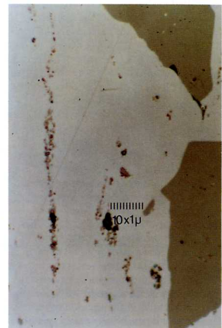
Figure 3c — Largest insoluble particles (excluding oxides) in 3% Ti-0.2% B (1000X)
