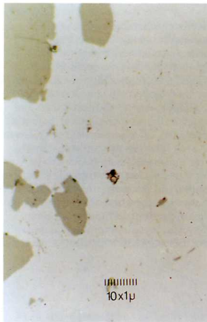
Figure 3b — Largest insoluble particles (excluding oxides) in 6% Ti-0.02% B (1000X)
